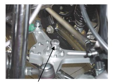
Anticlockwise turning: less damping Clockwise turning: more damping
