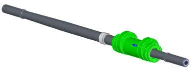
Balls of bearing drop in to circular groove Grease the bearings!
